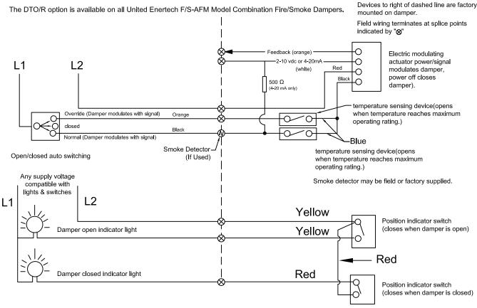
Switch is in Normal Position, damper motor is energized until thermostat senses temperature above initial closure rating. Above temperature closure rating, the damper motor is de-energized and damper closes.
